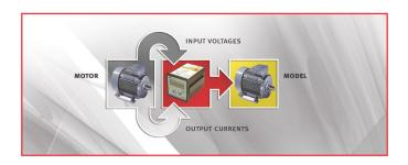
During learn mode Artesis MCM acquires real-time data from the physical equipment before applying advanced system identification algorithms to calculate a set of model parameters. The
